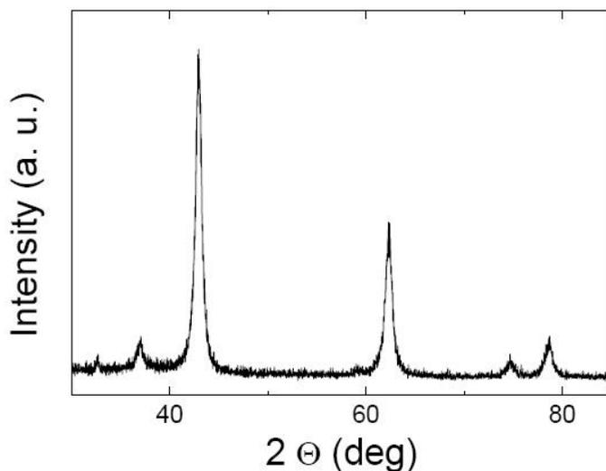
Figure 1. X-Ray diffraction pattern of nano-silicon dioxide particles.
