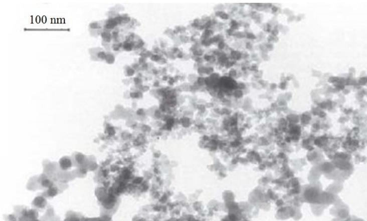
Figure 2. Large area TEM image of SiO<sub>2</sub> nano-particles.
